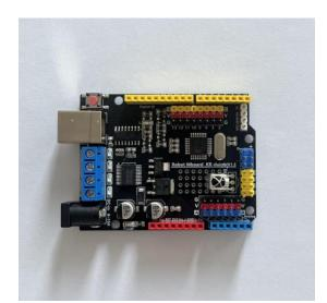
A type of microprocessor that integrates the functions of CPU (central processing unit) into a single chip. This reduces the need for additional components, making them more convenient. It interprets the EMG sensors and translates these signals into precise movements of the electronic device Despite its lower performance compared to a microprocessor, it is commonly used in simpler and smaller projects due to its compact design, flexibility, and ease of use.
