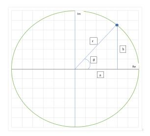
The diagram above presents a complex number on a complex plane. As shown in the graph above, the complex number creates a right-angled triangle on the complex plane.
