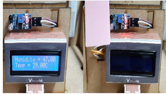
(a) (b) Figure 13. LCD backlight turns on or off based on obstacles (a) No obstacles (b) Obstacles present
